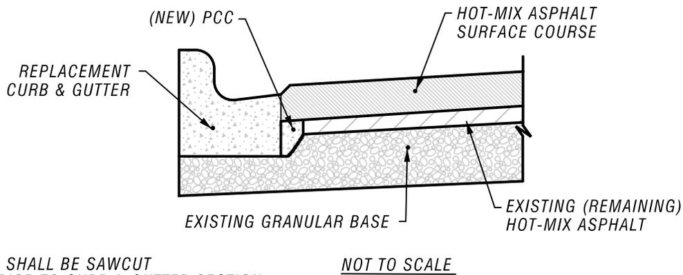
\* CURB & GUTTER SHALL BE SAWCUT (FULL DEPTH) PRIOR TO CURB & GUTTER SECTION.
